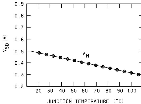
FIGURE 3161-5. Example curve of  $V_{SD}$  versus  $T_J$ .
