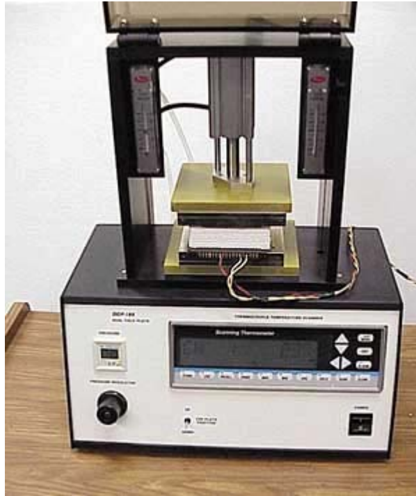
Figure 3. Test Setup: The DCP-100 dual cold plate test fixture set up for \theta_{JC} measurements using the bottom cold plate for heat sinking and the top cold plate as a pressure plate.
