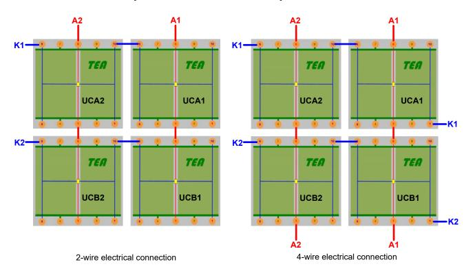
Using the matrix approach, only 4 connections in 2-wire configuration and 8 connections in 4-wire configuration are necessary to access four diodes. This compares to 8 and 16 connections, respectively, if each diode had separate individual connections.
