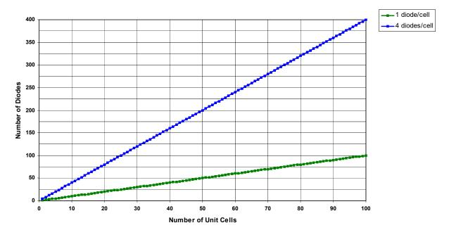
For the case of 2-wire electrical configuration, 200 electrical connections would be required for temperature measurements using 100 diodes. 400 electrical connections would be necessary for the 4-wire (Force & Sense) electrical configuration. In most cases, the number of electrical connections for either configuration can be reduced by sharing connections between diodes – for example, the cathodes for all diodes connected together.
