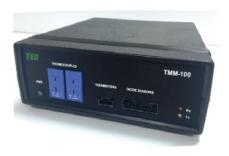
The internal precision  $I_M$  current source provides 1.00mA. Voltage compliance is 2V. The internal voltage measurement circuit provides measures to 1.999V with mV resolution for any of the selected eight diode temperature sensing channels. The diode voltage can be automated converted to temperature measurements using the software's built-in calibration capability. The temperature measurement resolution of 0.01°C for all sensors provides for accurate temperature differential measurements.
